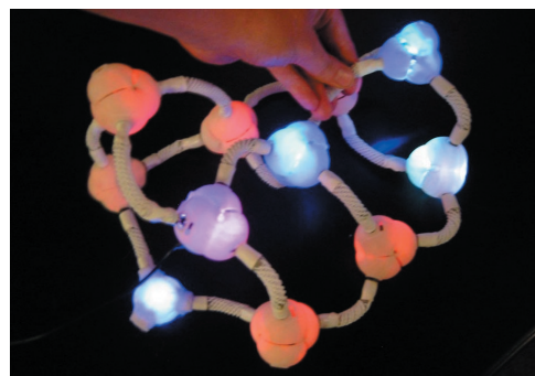
Figure 1. The Senspectra System: Tetrahedral Nodes and Sensor Joints
