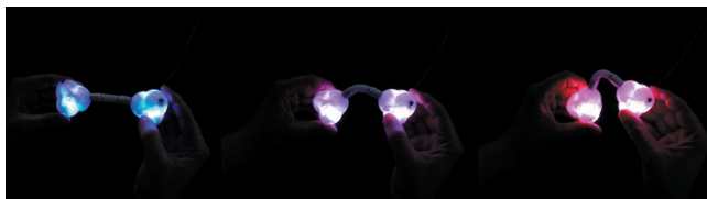
Figure 4. Nodes change color as the joint between them is bent.
